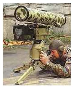
The operator uses either optical or thermal sight to detect and track the target. <a href="http://www.army-technology.com/projects/kornet/">http://www.army-technology.com/projects/kornet/</a>
